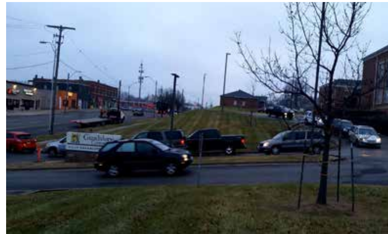
Figure 16. At its longest, queued traffic stretches eight to ten cars while drivers wait for gaps in traffic to turn left.
