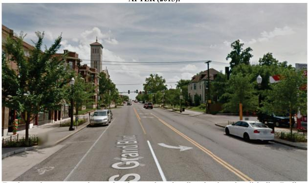
Two lanes plus center turn lane and parking, wider sidewalk and wider sidewalk buffer. Traffic is calmed and much slower (25 mph speed limit) so that separate bicycle facilities are not necessary in this section now
